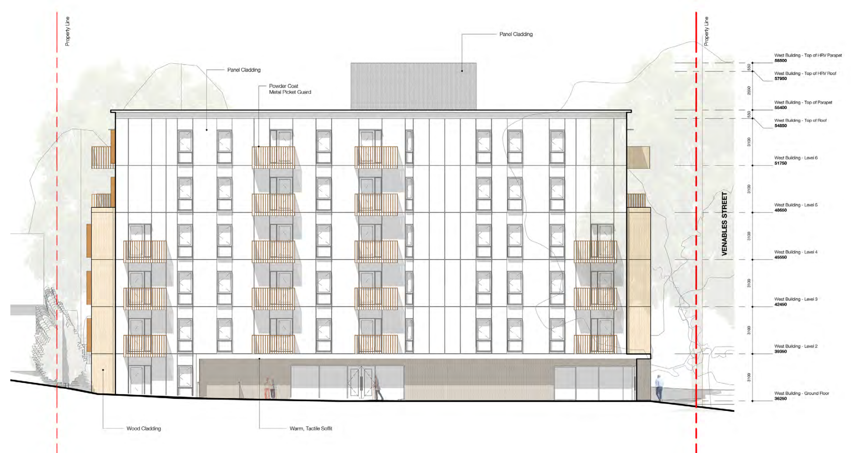
West Building – East Elevation
